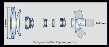
The wide-angle zoom lens that gained high popularity in the HVX200 Series has been reduced in size, lightened, and further widened in this 13x zoom lens. The new lens structure combines 13 lens elements in 10 groups, with 3 aspherical lenses. The diameter of the front lens element has been reduced from 67 to 53.2 mm, while still achieving a 28mm wide angle (35mm equivalent), the widest of the class.\*
